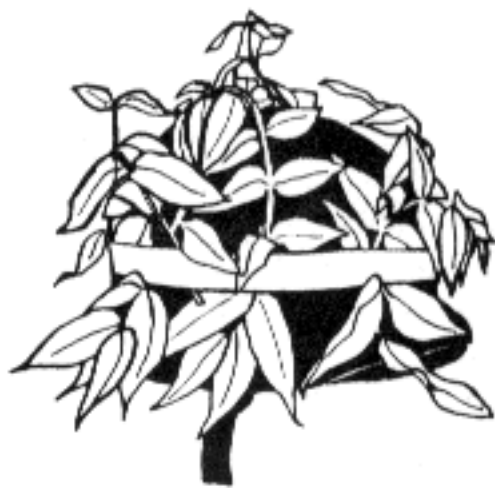
(1) Rubber bands, or expedient bands made from old inner tubes or burlap strips, secure natural materials. (Note position of band.)
